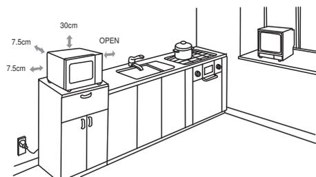
**A minimum clearance of 7.5cm is required between the oven and any adjacent walls. One side must be open.**
